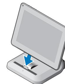
Align the computer with the docking station connector and press down until it clicks into place.
